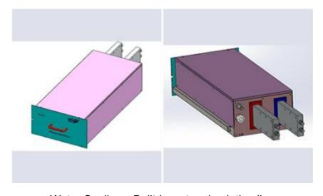
Water Cooling: Built-in water circulation line
